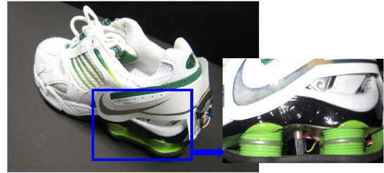
Fig. 6. Self-powered RFID shoe with mounted electronics.
