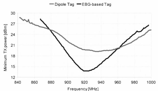
Fig. 4. Sensitivity analysis in anechoic chamber: comparison between EBG-based Tag and dipole Tag.
