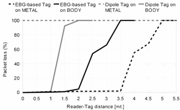
Fig. 5. Indoor read-range analysis: comparison between EBG-based Tag and dipole Tag attached to different surfaces.
