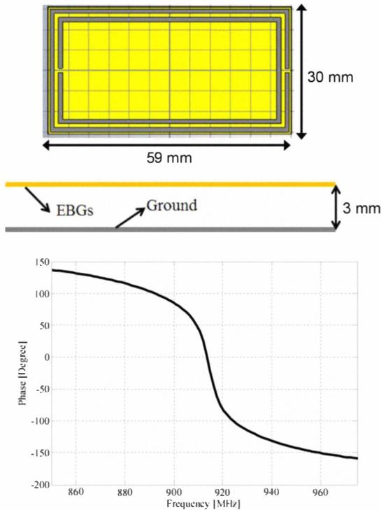
Fig. 1. EBG unit cell (top) and the resulting simulated reflection phase (bottom).
