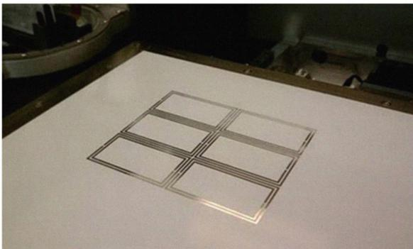
Fig. 2. Fabricated EBG structure by means of inkjet printing.
