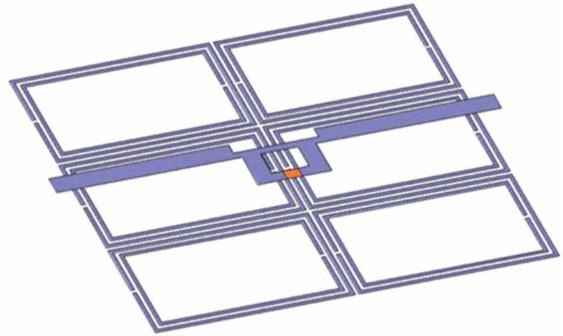
Fig. 3. Dipole antenna matched to the RFID chip on top of the designed SRR-based EBG surface.
