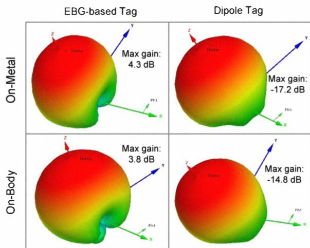
Fig. 6. Simulated 3D radiation patterns of the EBG-based and dipole Tags on both metal and body.
