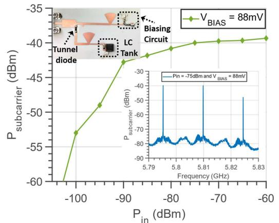
Fig. 6. Fabricated combined oscillator/reflection amplifier system on RO4003C with the measured sub-carrier powers over a range of RF input powers in addition to the display of the modulated and amplified RF signal for  $P_{in} = -75$  dBm.
