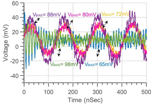
Fig. 2. Measured oscillations for the tunnel diode-based oscillator for different biasing conditions.
