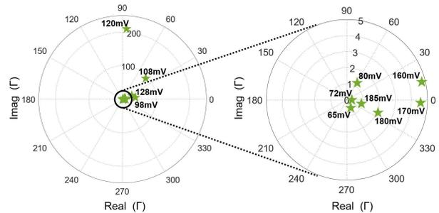
Fig. 3. Measured reflection coefficients  $\Gamma$  (real and imaginary components) for the reflection amplifier for different biasing voltages for an RF signal input power  $-75$  dBm and a frequency of 5.8 GHz.
