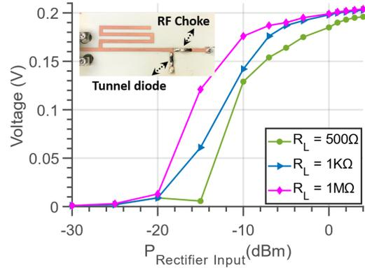
Fig. 5. Measured output voltages for the tunnel diode-based rectifier versus RF input powers for different load conditions.
