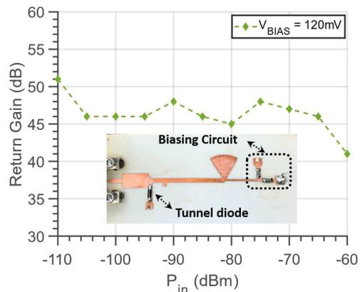
Fig. 4. Measured return gains for the reflection amplifier with respect to RF input powers for a biasing voltage of 120 mV and a frequency of 5.8 GHz.
