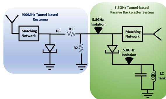
Fig. 1. Schematic of the fully-tunnel-diodes-based passive backscatter tag.
