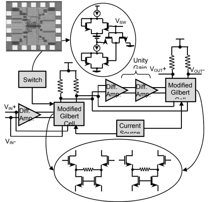
Fig. 5. Simplified schematic of  $360^\circ$  range controllable active phase rotator, and microphotograph of die.
