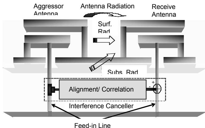
Fig. 2. Interference sources and cancellation mechanism.
