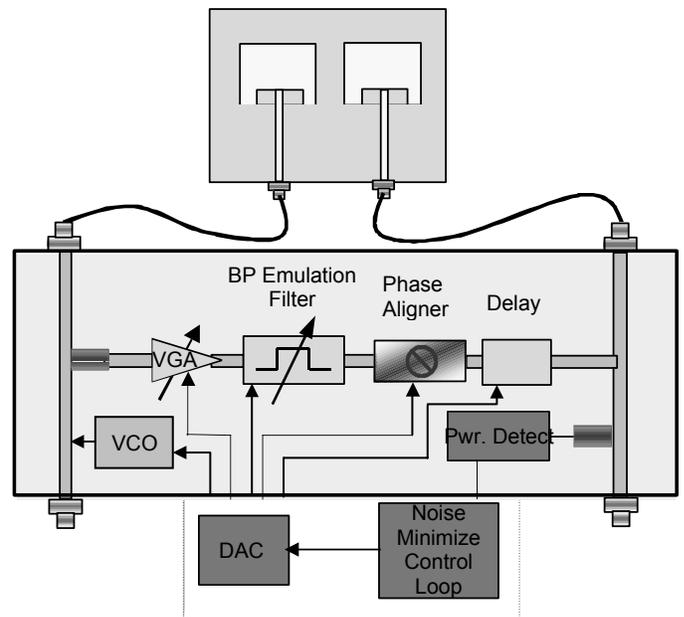
Fig. 3. Simplified schematic of interference canceller.
