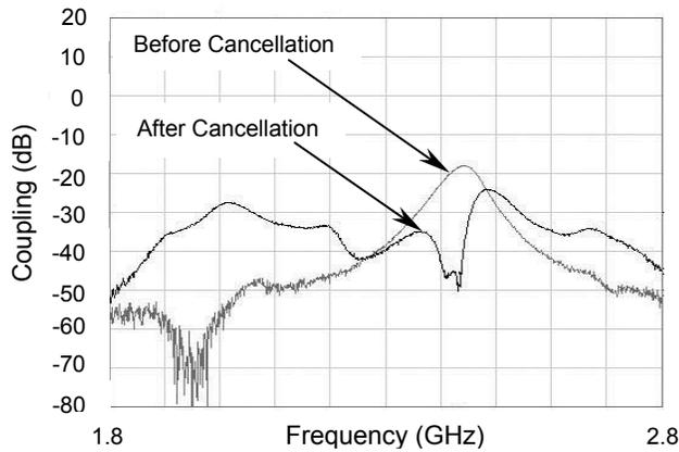
Fig. 6. Coupling spectrum before and after interference cancellation.
