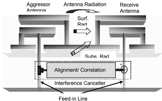
Fig. 2. Interference sources and cancellation mechanism.
