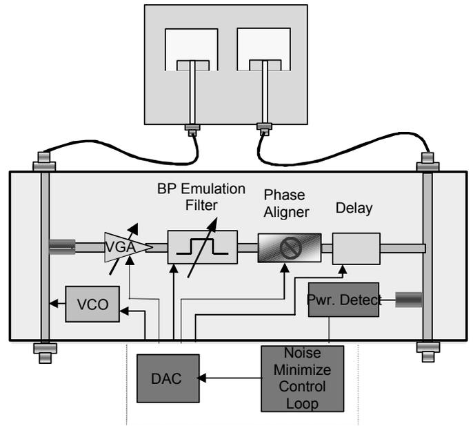
Fig. 3. Simplified schematic of interference canceller.
