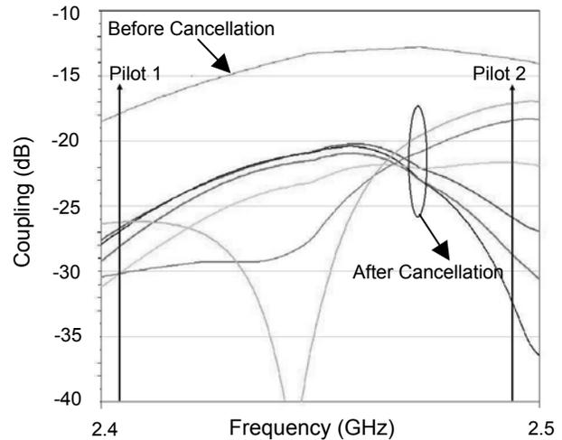
Fig. 8. Interference cancellation with the aid of two pilot tones for various phase adjustments in the correlation chain.
