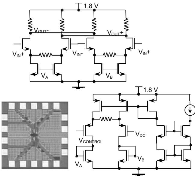
Fig. 4. Schematic circuit diagram of VGA and current source.
