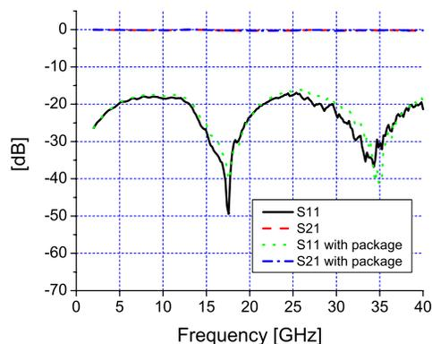
Fig. 7. Comparison of S-parameter measurements of the MEMS switch transmission line after the switch was physically removed. The cases with the package and without the package layer are nearly the same.
