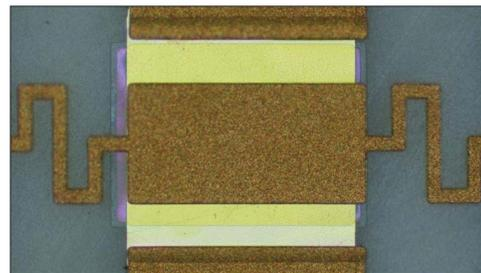
Fig. 4. Fabricated RF MEMS switch.
