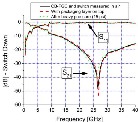
Fig. 6. Comparison of S-parameter measurements of an air-bridge type CB-FGC MEMS switch in the “DOWN” state. The three measurement cases shown are the same as those explained in the caption for Fig. 5.
