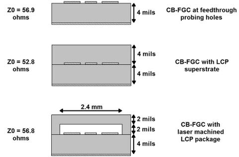
Fig. 1. Three different CB-FGC cross sections present in the measured packaging structures. Impedance values are from HFSS 3D simulator for an CB-FGC with signal width  $S=200 \mu\text{m}$ , gap  $G=120 \mu\text{m}$ , and  $\epsilon_r = 3.16$ .  $Z_0$  only differs by 4  $\Omega$  for the three different cross sections.
