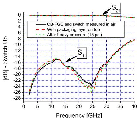
Fig. 5. Comparison of S-parameter measurements of an air-bridge type CB-FGC MEMS switch in the “UP” state. Case 1: The switch is measured in open air. Case 2: The packaging layer is brought down and taped into hard contact and measured. Case 3: A top metal press plate and a fifteen pound weight are put on top of the packaging layer (15psi) to simulate bonding pressure. The weight and the press plate are then removed and the switch is re-measured.
