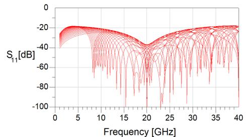
Fig. 2.  $S_{11}$  for cavities with electrical lengths from 0-360°. The CB-FGC in the cavity has  $Z_0 = 57 \Omega$  and the CB-FGC with superstrate feeding the cavity has  $Z_0 = 53 \Omega$ . The feeding CB-FGC lines are  $\lambda_G/4$  at 20 GHz which is an optimal configuration for minimizing the already low reflections.
