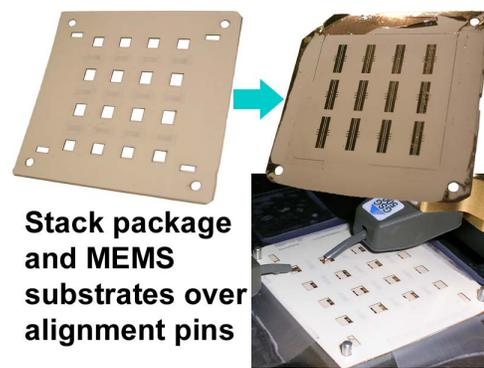
Fig. 3. Top left: LCP superstrate packaging layer with holes for alignment and probe feed-throughs. The packaged cavities between each set of probing holes are visible due to LCP becoming partially transparent at a 2 mil thickness. Top right: CB-FGC transmission lines with air-bridge RF MEMS switches in the center of the transmission lines. Bottom right: Both layers stacked on alignment fixture and probed through the feed-through windows.
