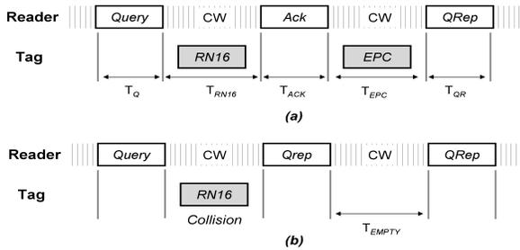
Figure 1. Gen2 protocol in case of single-Tag reply (a) and Tag collision (b).
