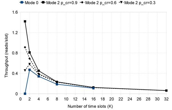
Figure 5. Measured throughput per slot ( $N=2$  tags) with three different values of collision-recovery probability set for the reader.
