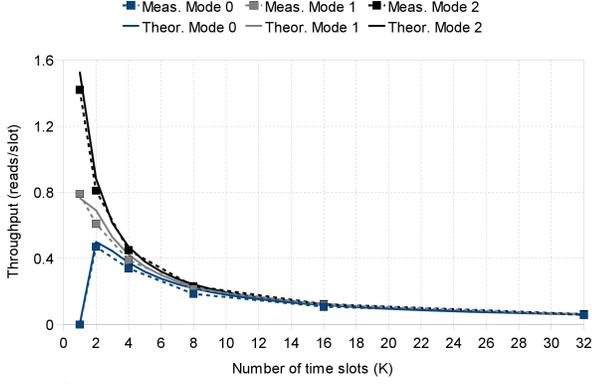
Figure 4. Comparison between theoretical and measured throughput ( $N=2$  Tags).
