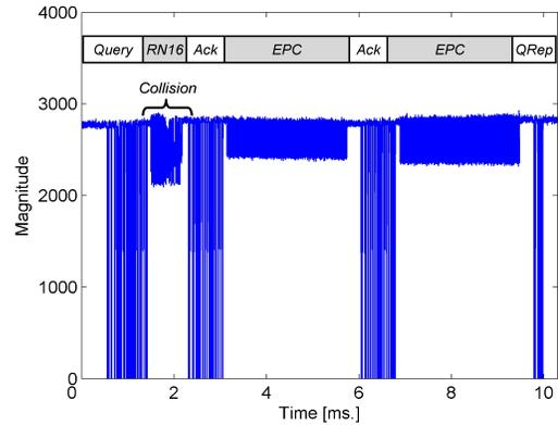
Figure 3. Example of captured Reader-WISPs communication with *Mode 2*.
