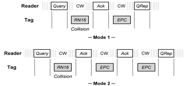
Figure 2. Proposed schemes for the EPC Gen2 MAC protocol in case of two-Tag collision recovery.
