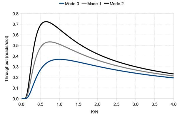
Figure 6. Expected throughput per slot with probabilities of collision detection and recovery set to 0.83 and 0.9, respectively.
