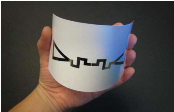
Figure 17. Photograph of the conformal tag with a single-walled nanotube film in the center.
