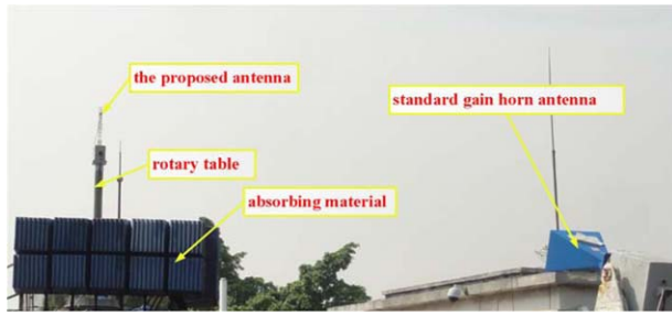
Figure 7 Photo of the measurement setup of the radiation patterns. [Color figure can be viewed in the online issue, which is available at wileyonlinelibrary.com ]
