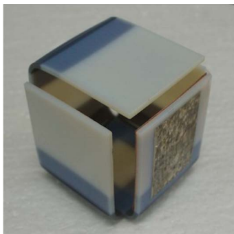
Fig. 21. Flexible 3-D printed SMA cube with an inkjet-printed antenna on one of its faces [38].
