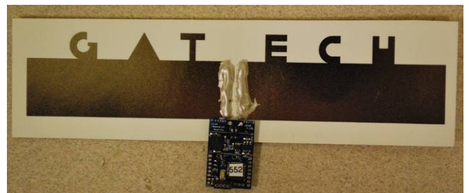
Fig. 5. Printed antenna mounted on the WISP.
