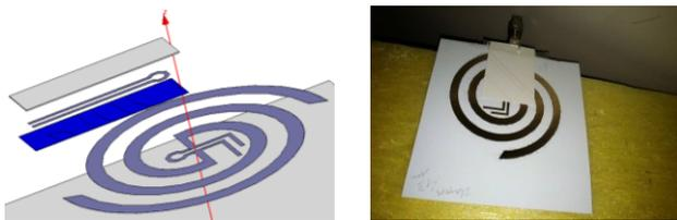
Fig. 7. (a) exploded view of the fabricated prototype. (b) capture of the fabricated prototype at 1.5 GHz range.
