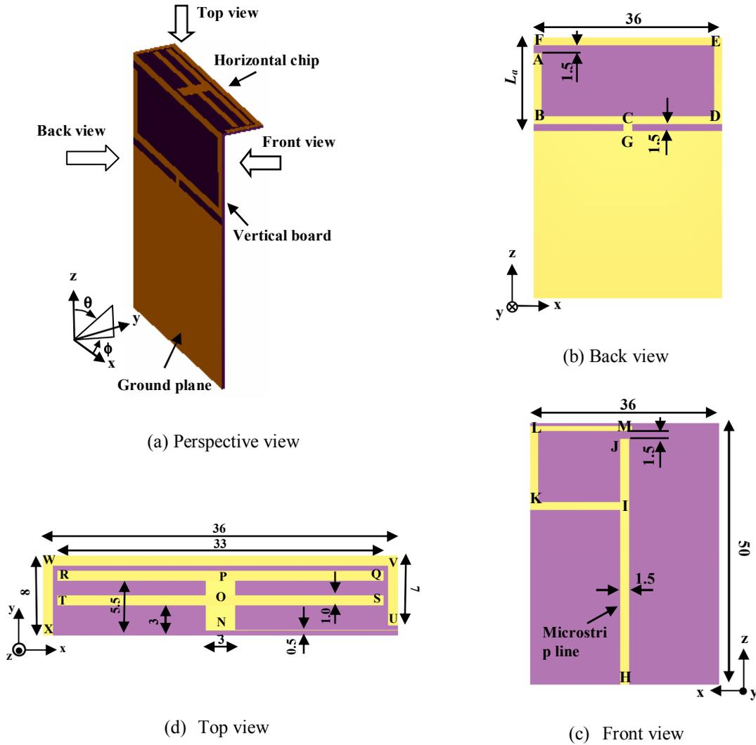
**Fig. 1 Configuration of a miniature broadband antenna (unit: mm)**
