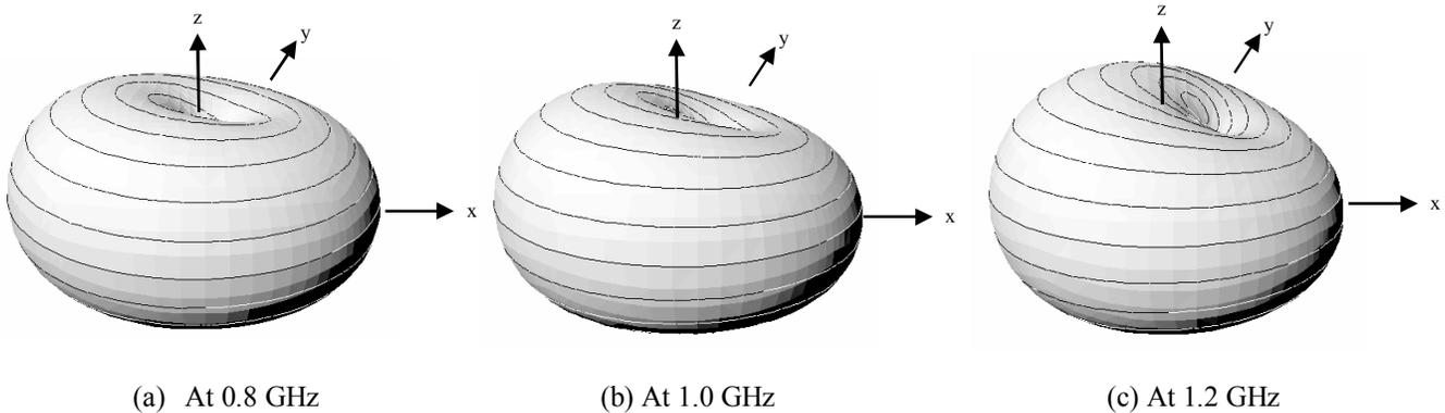
**Fig. 4 Radiation patterns of the miniature broadband antenna**
