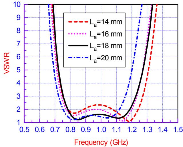
**Fig. 2 Dependence of the broadband performance on the antenna length ( $L_a$ ) on the vertical board**
