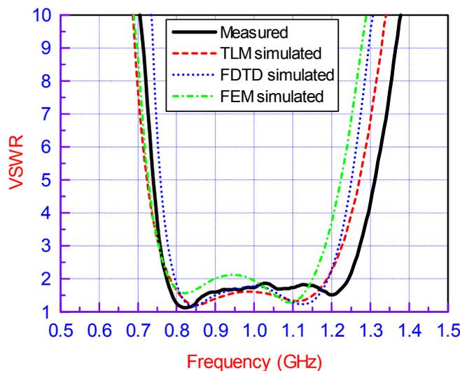
**Fig. 3 Comparison of measured and simulated results for the VSWR ( $L_a=18$  mm)**
