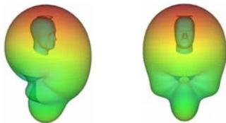
Figure 6. Metallic antenna on "SEP" Human Phantom (PEC  $\epsilon_r=1$ ).
