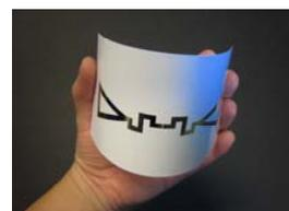
Figure 4. Photograph of the paper-based conformal tag.
