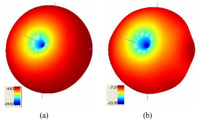
Figure 1. Measured radiation pattern of (a) the flat RFID tag and (b) the conformal RFID tag. Max gain drops from -4.63 to -7.37 dBi.
