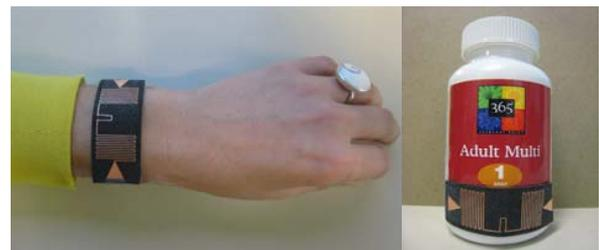
Figure 2. Embodiments of the conformal RFID tag prototype in the applications of wireless health monitoring and pharmaceutical drug bottle tracking.
