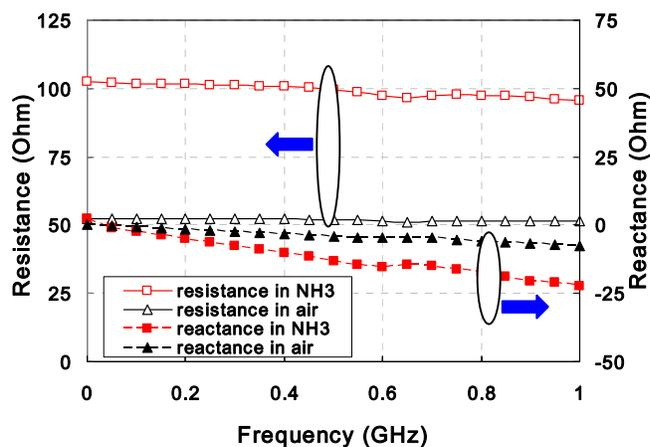
Figure 3. Measured electrical resistance of SWCNT gas sensors.
