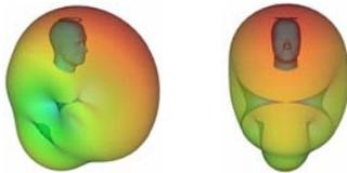
Figure 5. Liquid Antenna on "SEP" Human Phantom (NaCl  $\epsilon_r=40$ ,  $\tan \delta = 0.175$  @ 915 MHz).
