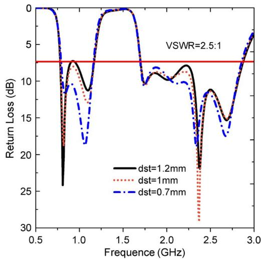
Fig. 3. Effect of the distance (dst) between the s-strip and invert-F strip on the return loss of the multiband planar antenna, where dst was changed from  $dst = 0.7\text{ mm}$  to  $dst = 1.2\text{ mm}$ . The optimized value for dst is  $\sim 0.7\text{ mm}$ .
