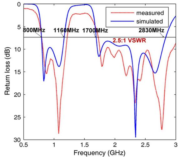
Fig. 6. Comparison between the measured and simulated result for return loss of the multiband planar antenna.
