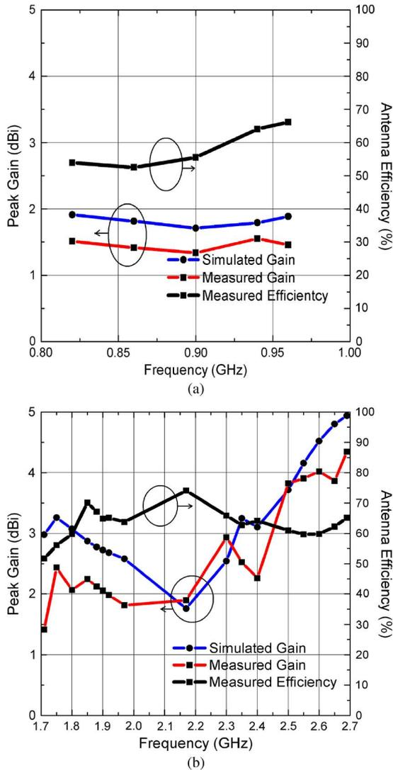
Fig. 8. Comparison between the measured and simulated results for peak gain of the multiband planar antenna and the measured antenna efficiency. (a) In lower band. (b) in higher band.
