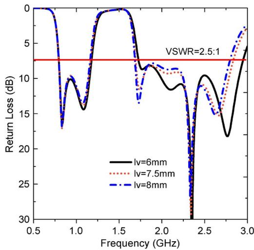
Fig. 4. Effect of the length (lv) of meandered strip on the return loss of the multiband planar antenna, where lv was changed from  $lv = 6\text{ mm}$  to  $lv = 8\text{ mm}$ . The optimized value for lv is  $\sim 7.5\text{ mm}$ .
