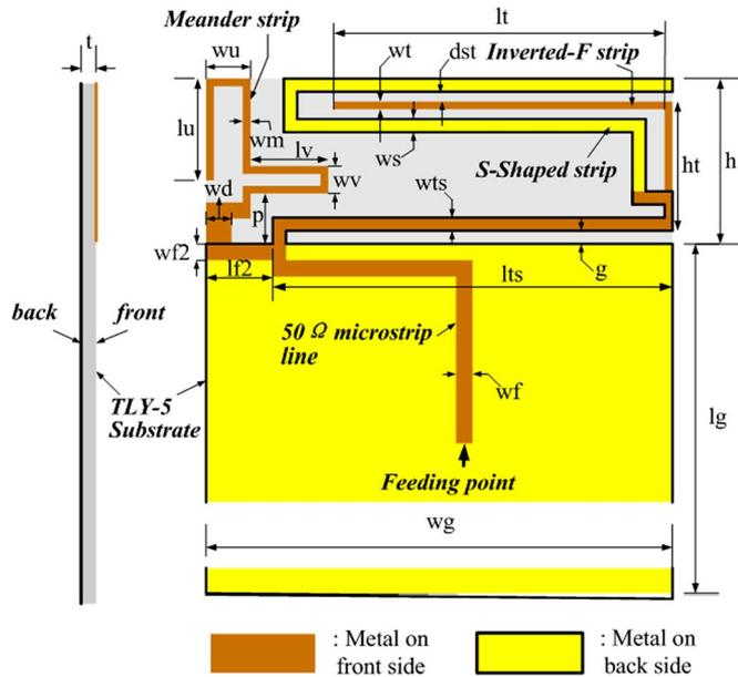
Fig. 1. Geometry of the multiband planar antenna which consists of a two-strip monopole for the 900-MHz band and a meandered strip for the 1900-MHz band.
