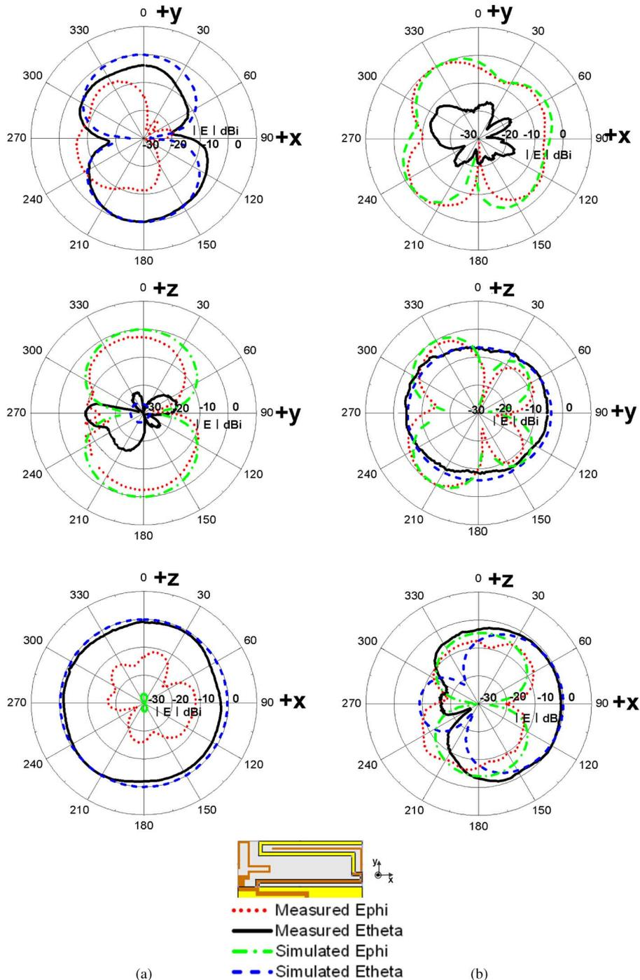
Fig. 7. Radiation patterns of the multiband planar antenna. (a) At 900 MHz. (b) at 1900 MHz.
