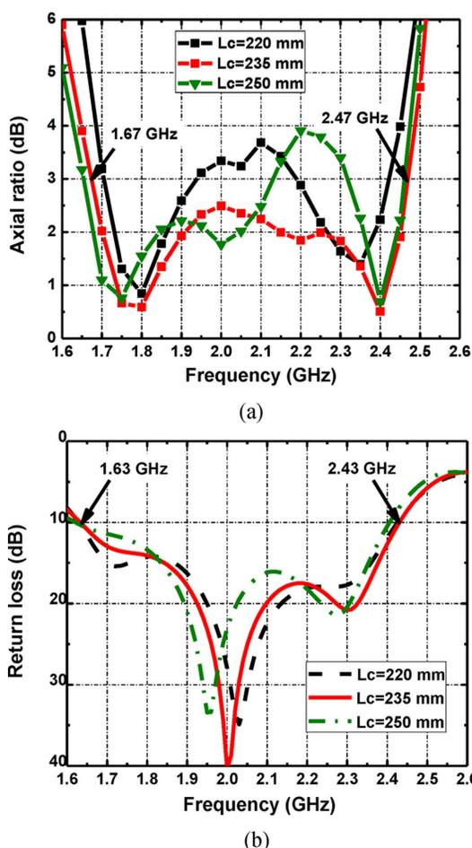
Fig. 6. Dependences of (a) axial ratio and (b) return loss of the omnidirectional CP antenna on the length of the conducting cylinder.
