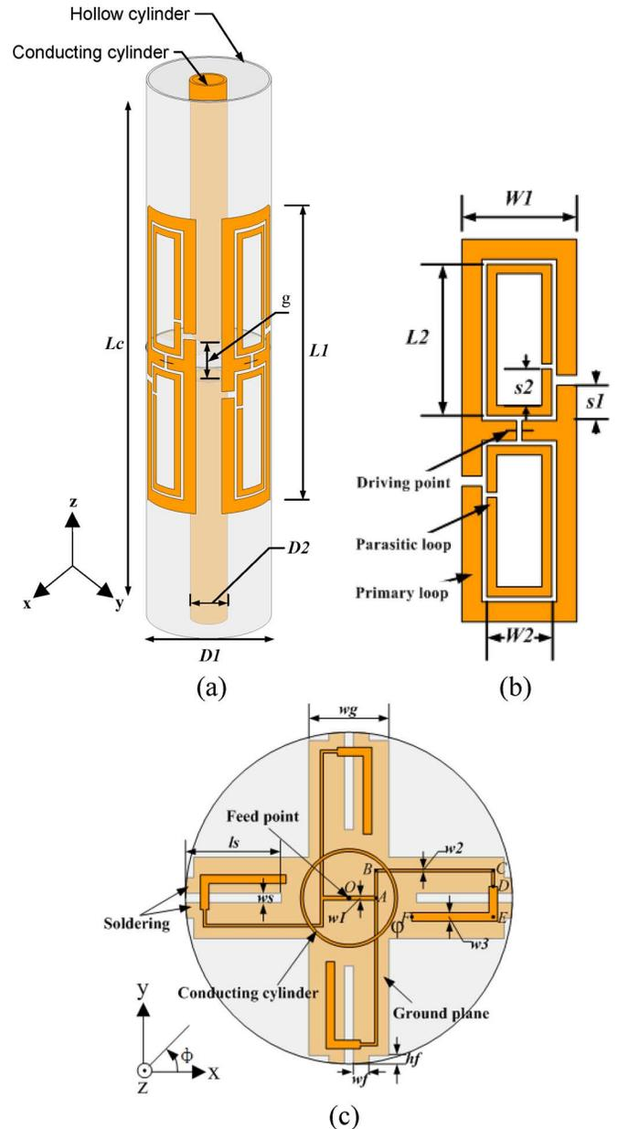
Fig. 1. Configuration of a broadband omnidirectional circularly polarized (CP) antenna: (a) perspective view; (b) broadband cp element; (c) feeding network.
