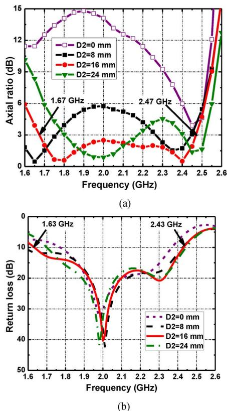
Fig. 5. Dependences of (a) axial ratio and (b) return loss of the omnidirectional CP antenna on the diameter of the conducting cylinder.
