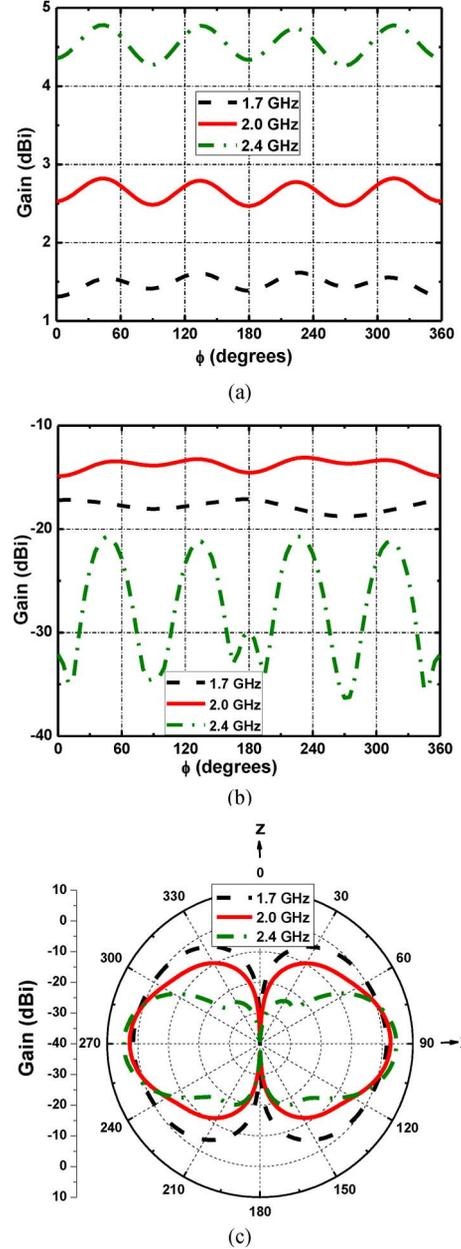
Fig. 3. Simulated gain patterns for the omnidirectional CP antenna: (a) LHCP in the horizontal plane (i.e., the  $xy$  plane); (b) RHCP in the horizontal plane (i.e., the  $xy$  plane); (c) LHCP in the elevation plane (i.e., the  $xz$  plane).
