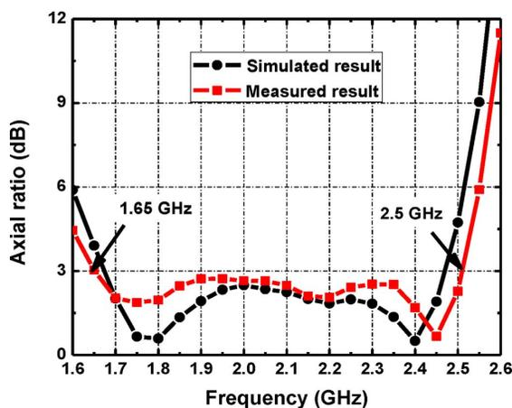
Fig. 11. Measured axial ratio for the omnidirectional CP antenna compared with simulation result.
