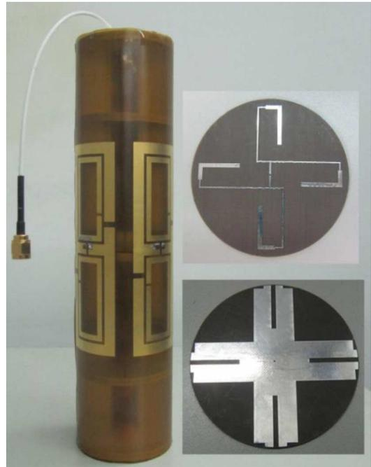
Fig. 9. Prototype of the broadband omnidirectional CP antenna with front and back views of the feeding network.
