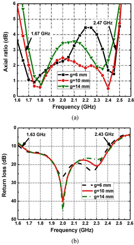
Fig. 7. Dependences of (a) axial ratio and (b) return loss of the omnidirectional CP antenna on the gap length of the conducting cylinder.
