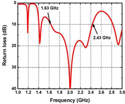
Fig. 2. Simulated return loss for the omnidirectional CP antenna.
