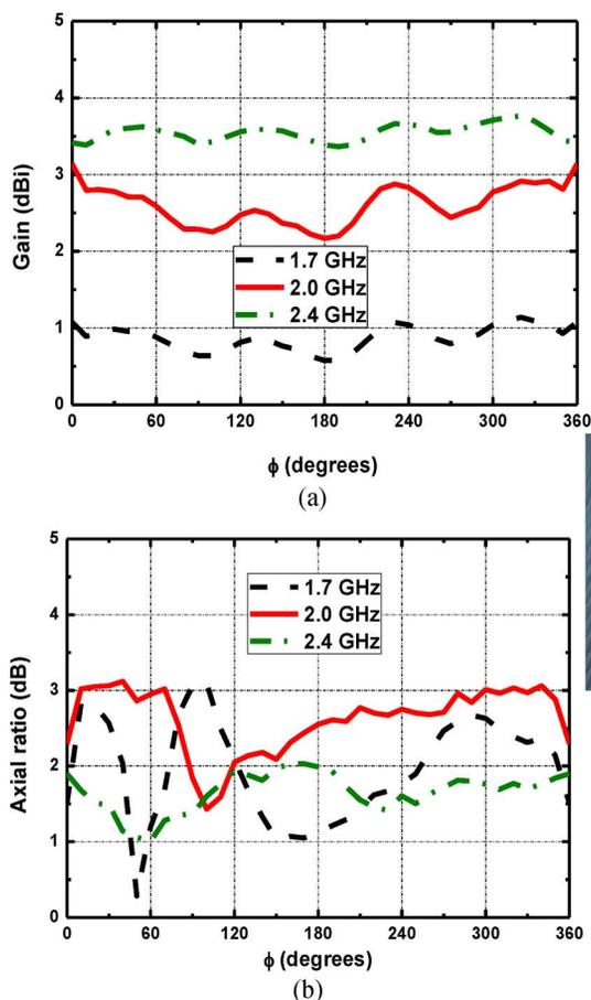
Fig. 13. Measured gain and axial ratio patterns for the omnidirectional CP antenna in the omnidirectional plane (i.e.,  $xy$  plane): (a) gain pattern; (b) axial ratio pattern.
