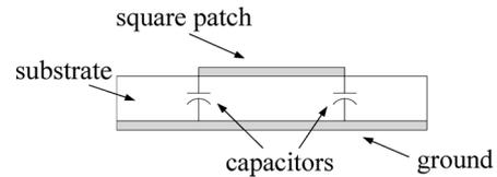
Fig. 4. Illustration of a microstrip antenna with tuning capacitors.
