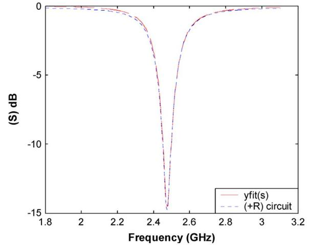
Fig. 3. S-parameter plot comparing the fitted function ( $y_{\text{fit}}(s)$ ) and the positive resistance equivalent circuit (1st row) and its magnitude deviation (2nd row) of patch antenna at around the 2.4 GHz band.
