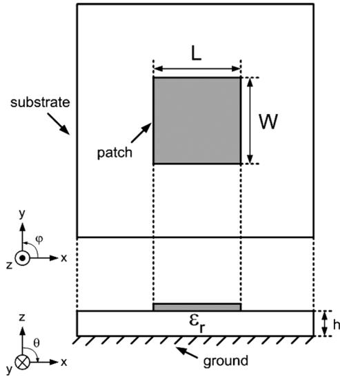
Fig. 2. Illustration of simple microstrip antenna.
