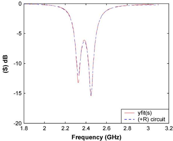
Fig. 5. S-parameter plot comparing  $y_{fit}(s)$  and the positive resistance equivalent circuit (1st row) and its magnitude deviation (2nd row) of the design in Fig. 4.
