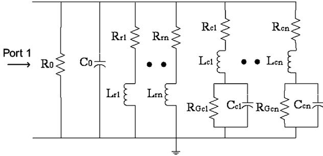
Fig. 1. Schematic of single-port equivalent circuit representation.
