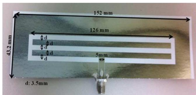
Fig. 1. Folded slot antenna geometry (gap of the CPW line: 0.2 mm).
