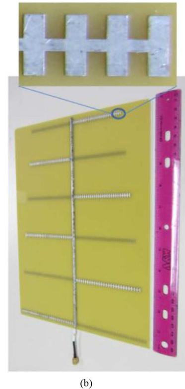
Fig. 4. (a) E-WEHP log periodic antenna structure dimensions. (b) E-WEHP log periodic antenna prototype fabricated on 0.062-in FR-4.
