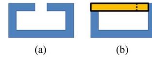
Fig. 3. Top view of the traditional and modified loops. (a) Traditional open loop. (b) Modified open loop.
