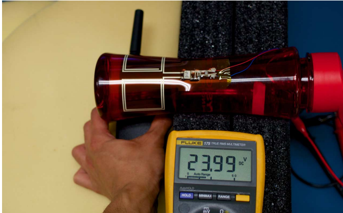
Fig. 19. Open voltage measurement of the conductive inkjet-printed H-field harvester with an on-bottle setup.
