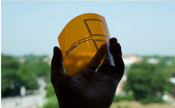
Fig. 4. Printed harvester circuit traces under bent/flex conditions.
