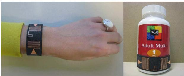
Fig. 10. Embodiments of the conformal RFID tag prototype in the applications of wireless health monitoring and pharmaceutical drug bottle tracking.
