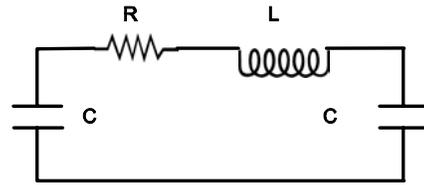
Figure 7: Equivalent circuit model of thin film resistor in FGC waveguide.
