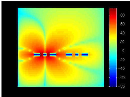
**Figure 17: Horizontal electric field component of coupled FGC waveguides ( $S=W=25\ \mu\text{m}$ ,  $B=50\ \mu\text{m}$ ,  $D=75\ \mu\text{m}$ ).**
