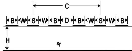
Figure 12: Coupled FGC waveguides.
