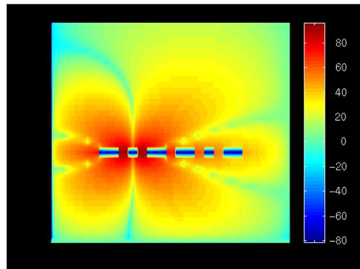
Figure 16: Horizontal electric field component of coupled FGC waveguides ( $S=W=25 \mu\text{m}$ ,  $B=50 \mu\text{m}$ ,  $D=25 \mu\text{m}$ ).
