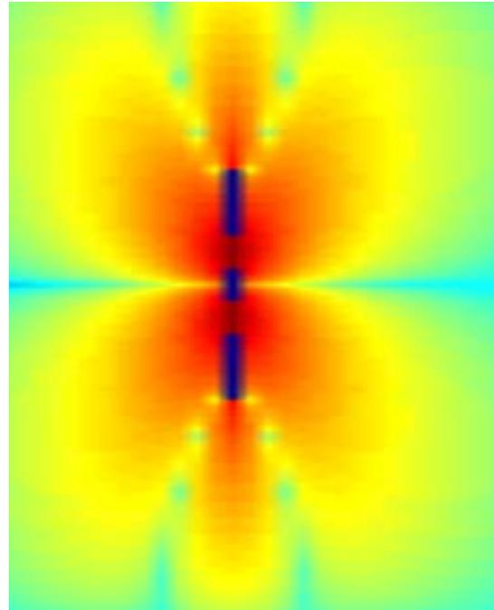
Figure 15: Horizontal electric field component of FGC waveguide ( $S=W=25 \mu\text{m}$ ,  $B=50 \mu\text{m}$ ).
