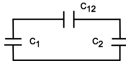
Figure 8: Equivalent circuit model of MIM capacitor in FGC waveguide.
