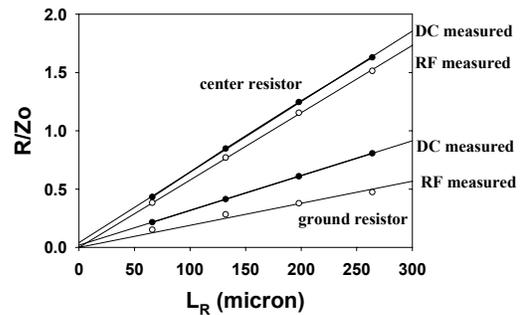
Figure 9: Measured resistance values of thin film resistor in FGC waveguide as a function of the resistor length.
