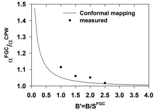
**Figure 4: Attenuation of FGC waveguide with  $S=W=25 \mu\text{m}$  normalized to the attenuation of conventional CPW with  $S=W=25 \mu\text{m}$  as a function of the normalized ground plane width.**
