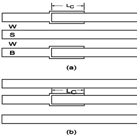
Figure 6: Schematic of MIM capacitor in the (a) ground planes and (b) center conductor of FGC waveguide.
