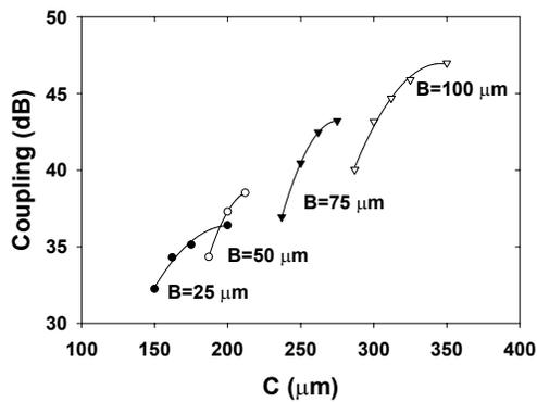
Figure 14: Measured coupling between FGC waveguides as a function of  $B$  and  $C$  ( $S=W=25 \mu\text{m}$ ).
