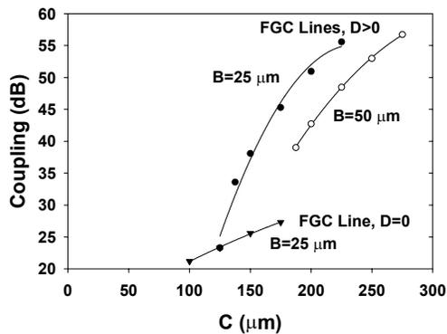
Figure 13: Coupling between FGC waveguides with  $D>0$  and between FGC waveguides with a continuous ground plane ( $D=0$ ) as a function of  $B$  and  $C$  determined by a 2D-FDTD analysis ( $S=W=25 \mu\text{m}$ ).
