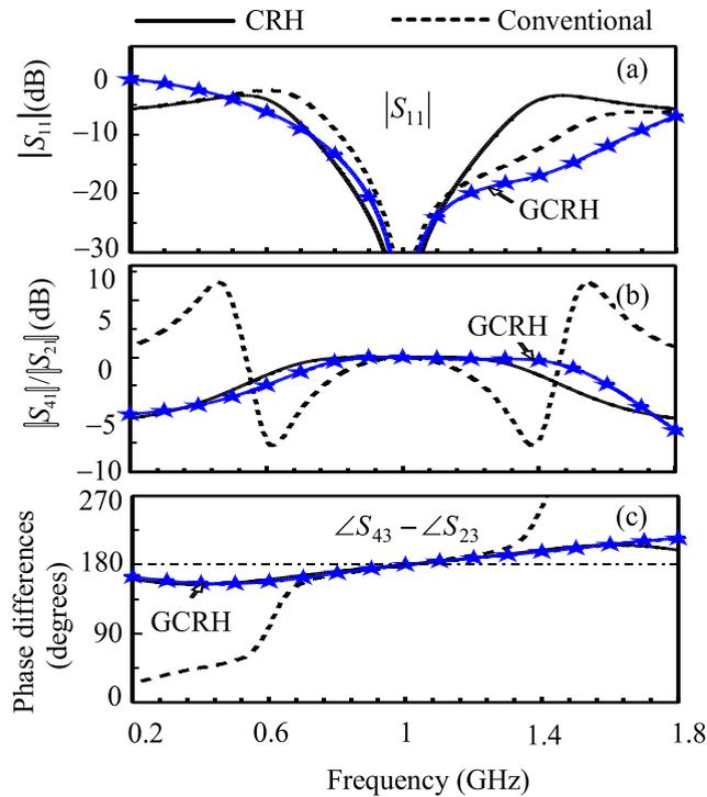
**FIGURE 5.** Compared frequency responses for  $k^2 = 0$  dB. (a)  $|S_{11}|$ . (b) Power-division ratios of  $|S_{41}|/|S_{21}|$ . (c) Out-of-phase responses of  $\angle S_{43} - \angle S_{23}$ .
