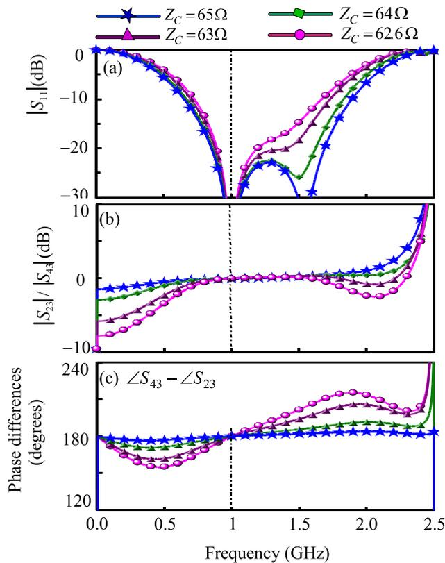
FIGURE 4. Frequency responses of GCRHs with  $C_{ap} = 0$  for  $k^2 = 0$  dB. (a)  $|S_{11}|$ . (b) Power-division ratios of  $|S_{23}| / |S_{43}|$ . (c) Out-of-phase responses of  $\angle S_{43} - \angle S_{23}$ .
