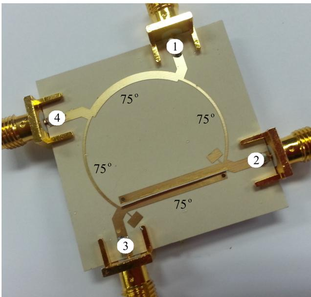
**FIGURE 9.** Fabricated prototype II (GCRHC) for  $k^2 = -5$  dB.
