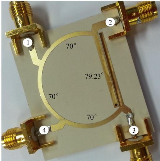
FIGURE 7. Fabricated prototype I (GCRH) for  $k^2 = 0$  dB.
