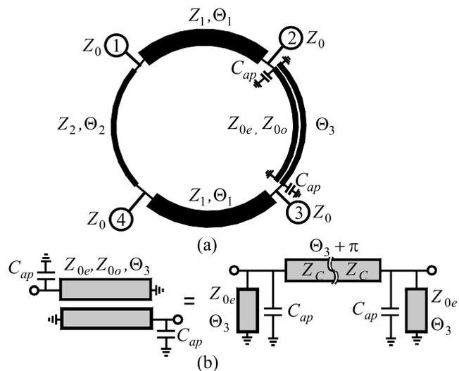
FIGURE 1. (a) GCRH topology. (b) Equivalent circuit of the CPL between ports ② and ③.
