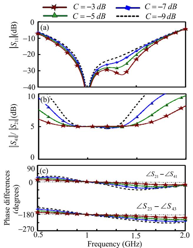
**FIGURE 6.** Frequency responses of GCRHCs for  $k^2 = -5$  dB. (a)  $|S_{11}|$ . (b) Power-division ratios of  $|S_{41}|/|S_{21}|$ . (c) In- and out-of-phase responses.
