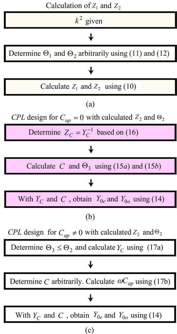
FIGURE 3. Design process for GCRHs. (a) Calculation of  $Z_1$  and  $Z_2$ . (b) CPL design for  $C_{ap} = 0$ . (c) CPL design for  $C_{ap} \neq 0$ .
