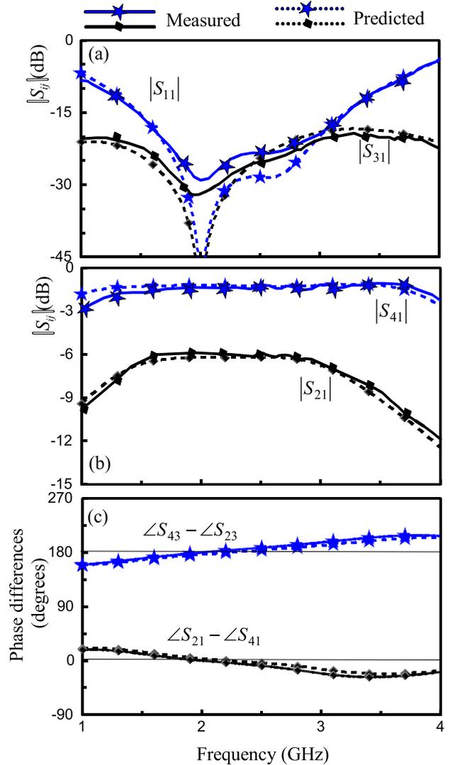
**FIGURE 10.** Measured and predicted frequency responses of prototype II (GCRHC) for  $k^2 = -5$  dB. (a)  $|S_{11}|$  (matching) and  $|S_{31}|$  (isolation). (b) Power divisions of  $|S_{21}|$  and  $|S_{41}|$ . (c) In- and out-of-phase responses.
