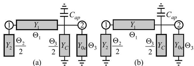
FIGURE 2. (a) Even-mode equivalent circuit. (b) Odd-mode equivalent circuit.
