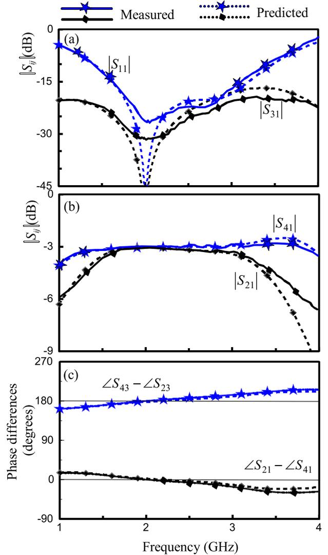
FIGURE 8. Measured and predicted frequency responses of prototype I (GCRH) for  $k^2 = 0$  dB. (a)  $|S_{11}|$  (matching) and  $|S_{31}|$  (isolation). (b) Power divisions of  $|S_{21}|$  and  $|S_{41}|$ . (c) In- and out-of-phase responses.
