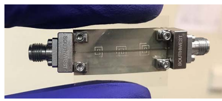
Fig. 1. (a) Design of the microfluidic RFID sensor, (b) Fabricated sample (front), and (c) Fabricated sample (back).
