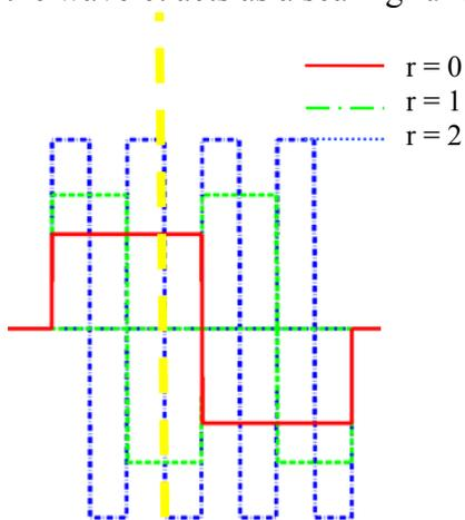
Fig. 3 Metal intersecting the center of a Haar MRTD cell
