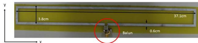
Fig. 2. Physical dimension of folded dipole antenna
