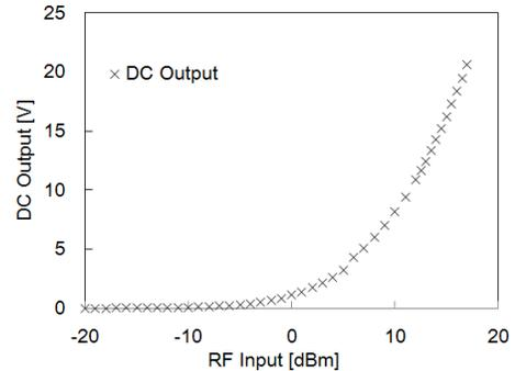
Fig. 5. DC output voltage of RF-DC charge pump circuit for different input power levels
