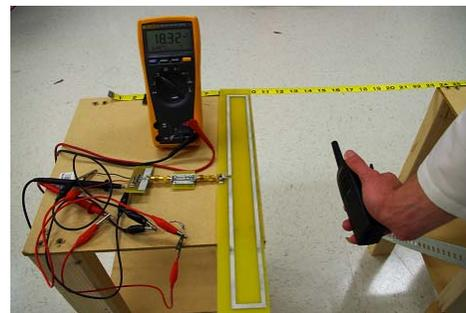
Fig. 6. Prototype harvesting ambient wireless power from a Motorola RDU2020 radio 13 cm away and giving 18.32V DC output voltage across 1 M-ohm load .
