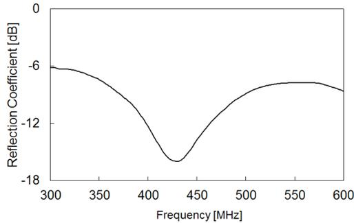
Fig. 3. Reflection coefficient of folded dipole antenna from 300 to 600 MHz
