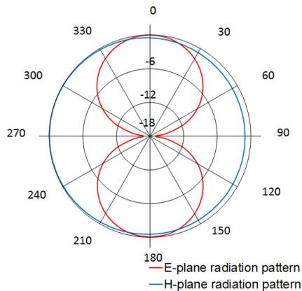
Fig. 4. E-plane and H-plane radiation pattern of folded dipole antenna
