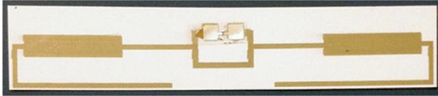
Fig. 2. Inkjet-printed IC-loaded antenna.
