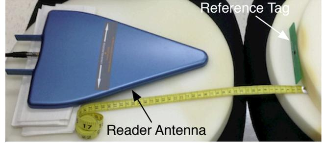
Fig. 3. Measurement setup. The calibration tag is shown at the same position that the tag under test is measured.
