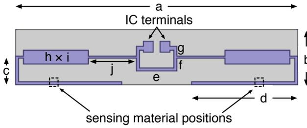
Fig. 1. Antenna layout.
