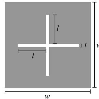
Fig. 1. (a) Unit cell for periodic cross-shaped slot FSS designed for 77 GHz with dimensions:  $w = 1.9$  mm,  $l = 1.4$  mm, and  $t = 0.1$  mm.
