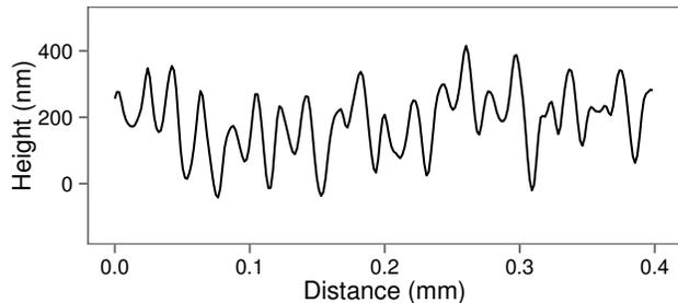
Fig. 3. Profilometer measurement of a 3D-printed SLA encapsulation surface.
