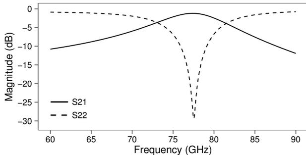
Fig. 2. S-parameter simulations of cross-shaped slot FSS unit cell.
