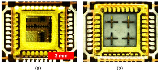
Fig. 4. Proof-of-concept 3D-printed SLA encapsulations for wireless IC packaging: (a) bare encapsulation and (b) inkjet-printed FSS-integrated encapsulation.
