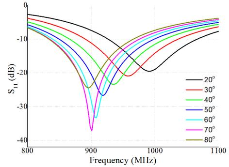
Fig. 2.  $S_{11}$  of the bowtie antenna for various apex angles.
