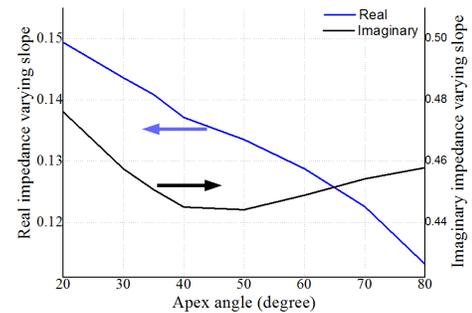
Fig. 3. The slope, variance of the real part and imaginary part of the antenna input impedance per frequency ( $\Omega$ /MHz), at the frequency of zero imaginary impedance for various apex angles.
