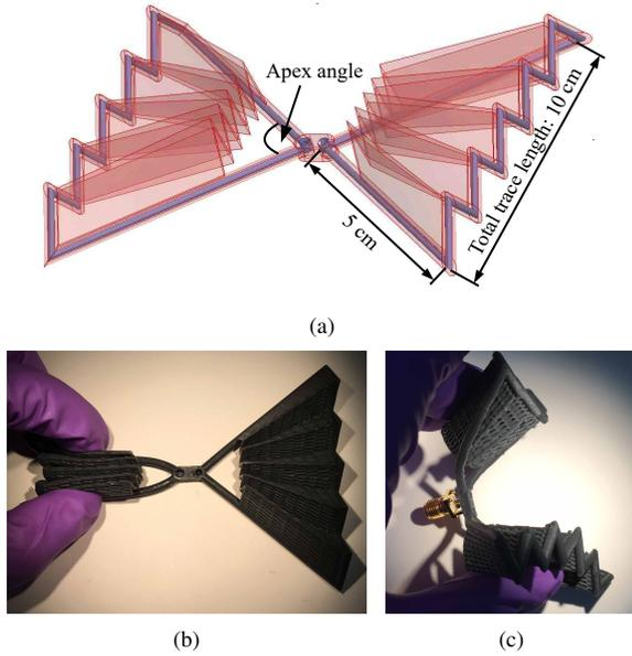
Fig. 1. Geometry (a) and photographs of a prototype (b, c) of the proposed “Chinese fan” bow-tie origami antenna. In (a), the red part is the 3D printed origami structure and the blue part stands for the microfluidic channel to contain LMA. In (b), the right fan is in its original state with a 80 degree apex angle and the left fan is compressed by two fingers to achieved a 30 degree apex angle. In (c), the antenna is folded up to show the flexibility.
