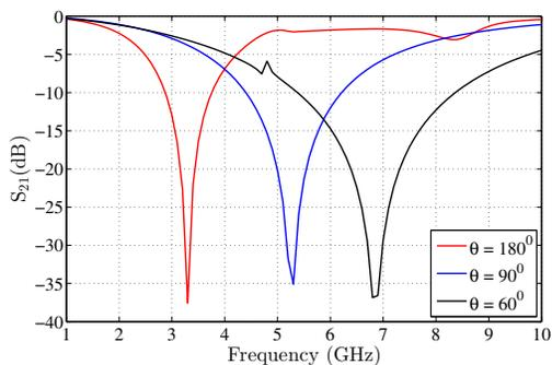
Fig. 3: Frequency response of 5-RiM FSS structure for different values of folding angle  $\theta$ .
