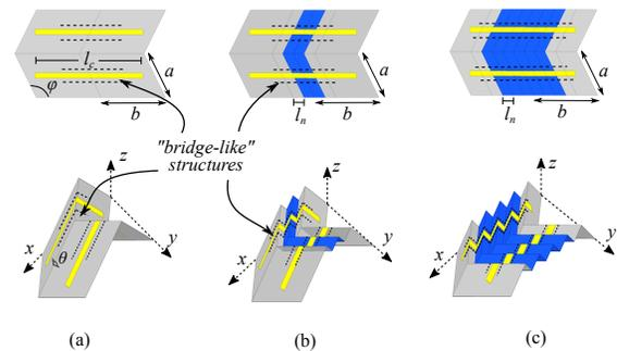
Fig. 1: Unit cell of (a) Miura (b) 3-RiM (c) 5-RiM FSS structure in flat (top) and folded (bottom) configuration.  $a=20\text{mm}$ ,  $b=30\text{mm}$ ,  $\phi=75^\circ$ ,  $l_c=50\text{mm}$  and  $l_s=5\text{mm}$ .
