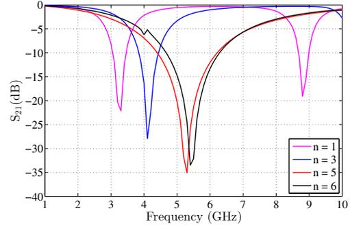
Fig. 4: Frequency response of n-RiM FSS structure for different number of ripples ( $n$ ) with  $\theta=90^\circ$ .
