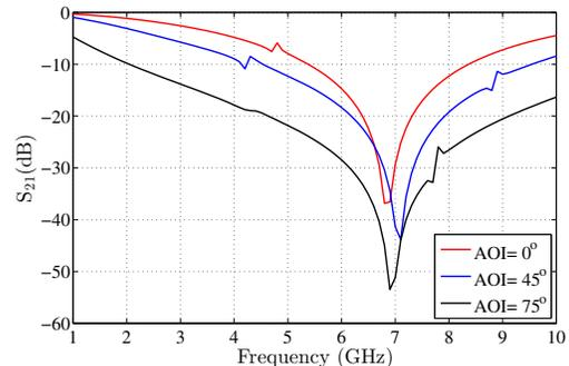
Fig. 5: Frequency response of 5-RiM FSS structure for different values of angle of incidence with  $\theta=60^\circ$ .
