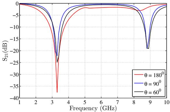
Fig. 2: Frequency response of Miura-FSS structure for different values of folding angle  $\theta$ .
