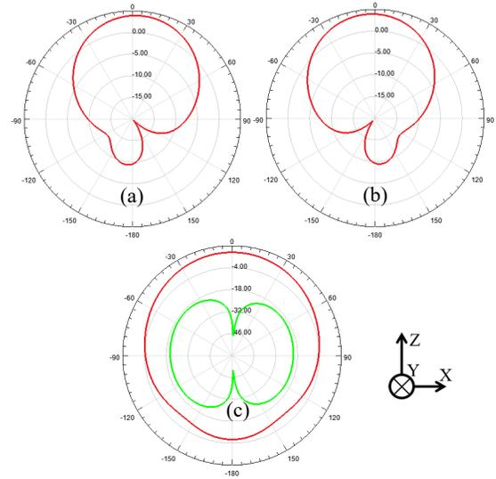
Fig. 3 Radiation patterns for (a) LHCP, (b) RHCP and (c) LP (and its x-pol)
