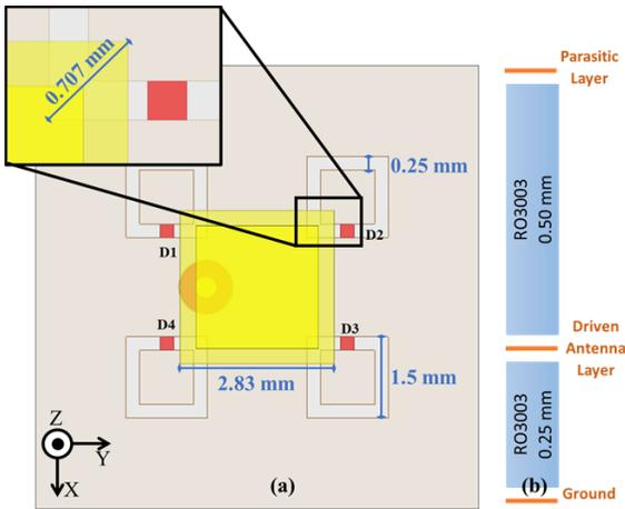
Fig. 1 (a) Layout's top view. (b) Illustrative side view.
