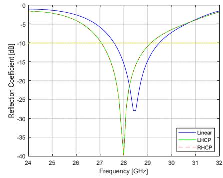
Fig. 2 Reflection coefficients for the LP and CP cases
