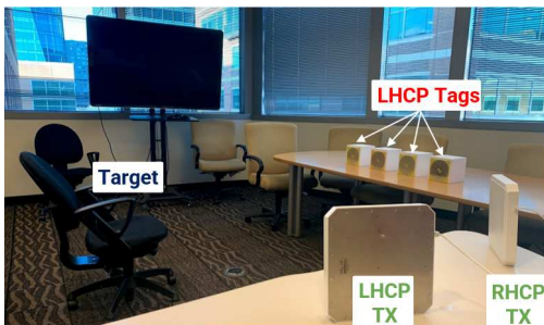
Fig. 2. Photo of the setup implementing four-tags linear array for target DOA estimation and BR extraction.
