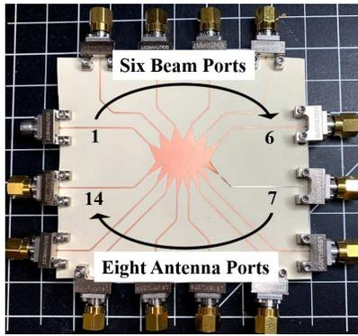
Fig. 1. Picture of the fabricated Rotman lens structure on thin LCP substrate.
