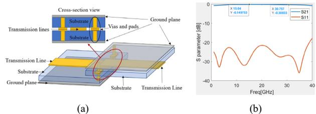
Fig. 1 Microstrip transition structure. (a) 3D schematic and cross section view (b) Simulation result of insertion loss
