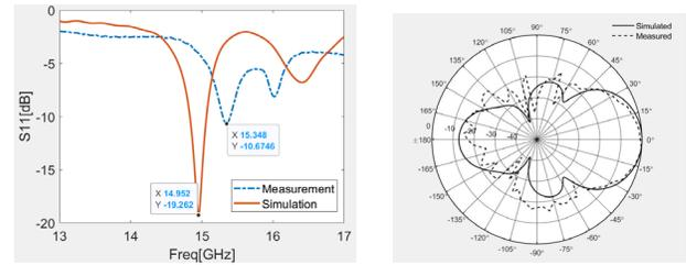
Fig. 3. Measured and simulated results of S11 and radiation pattern
