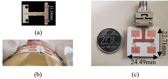
Fig. 2 Fabricated array tiles. (a) Basic feedline structure (b) Demonstration of flexibility (c) Size comparison for a 2 by 2 array
