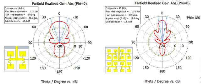
Fig. 4. Realized gain of a 4 tile array and a 16 tile array in simulation
