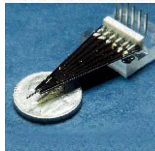
The probe is on 40 μ m-thick silicon mounted on a low resistivity 500 μ m-thick silicon wafer with a silver-epoxied low frequency connector on the right.
