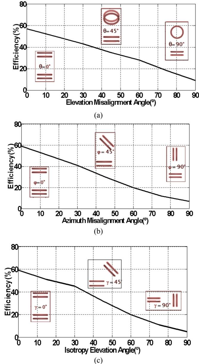
**Figure 2.** Standard SCMR under different misalignment conditions. (a) angular elevation, (b) angular azimuth, and (c) isotropy elevation.
