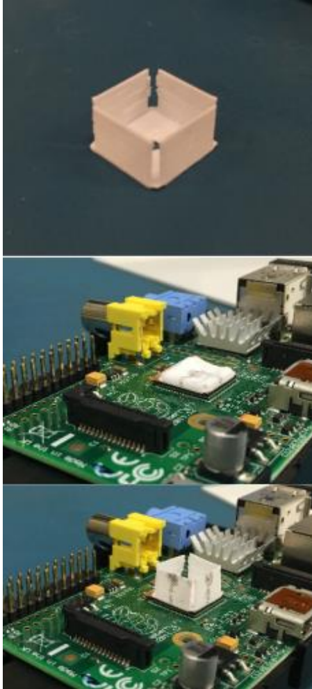
Figure 9. Shape Memory Polymer in permanent (top) state, temporary (middle), and recovery to permanent (bottom) states after SoC activity.
