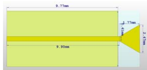
Figure 3. Simulation of 3D printed trapezoidal monopole antenna.
