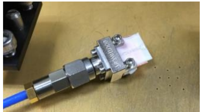
Figure 11. Single Antenna with Southwest Microwave Connector for S-parameter measurements.
