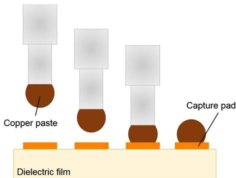
Fig. 8. Pin transfer assembly with a  $80\text{-}\mu\text{m}$  pin for transferring copper paste onto  $100\text{-}\mu\text{m}$  landing pads.
