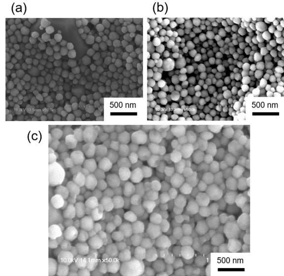
Fig. 5. SEM images of the copper paste B sintered for 30 minutes at (a) 200°C, (b) 230°C, and (c) 260°C.
