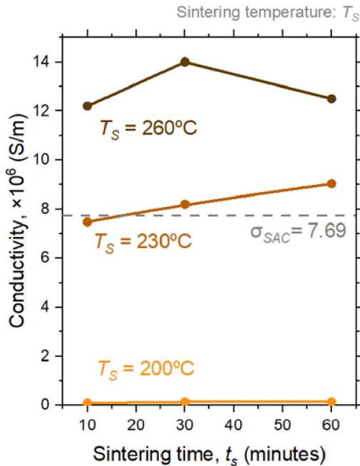
Fig. 4. Measured conductivity of the copper paste B with various sintering time and temperature annealed in the nitrogen gas.
