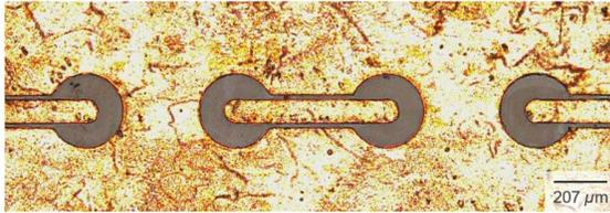
Fig. 7. Top view of the fabricated test vehicle with CPWG and landing pads for flip-chip assembly.
