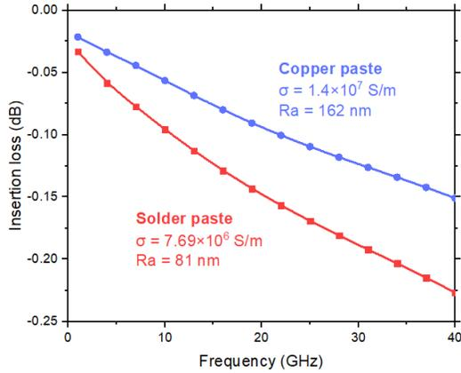
Fig. 10. Insertion loss as a function of frequency, computing the measured conductivity and surface roughness of the copper paste B and solder paste in the form for SAC305.
