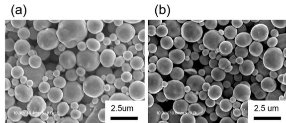
Fig. 3. SEM images of the copper paste A after sintering for 30 minutes at (a) 200°C and (b) 230°C.
