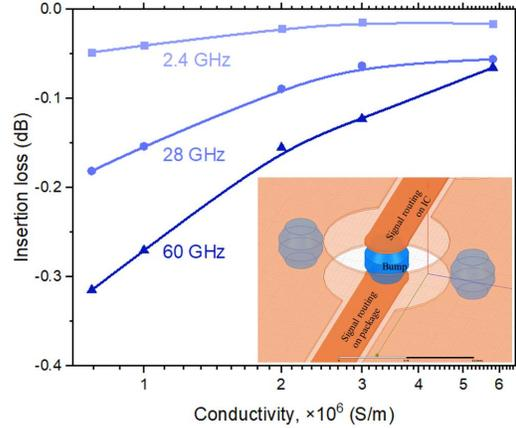
Fig. 2. Insertion loss in interconnect bumps at widely-used frequency bands for RF and 5G/mm-wave applications.
