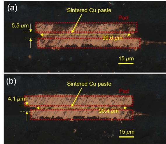
Fig. 9. Cross sectional images through optical microscope at two different locations of the assembled test vehicle with the copper paste B sandwiched by  $100\text{-}\mu\text{m}$  copper landing pads.
