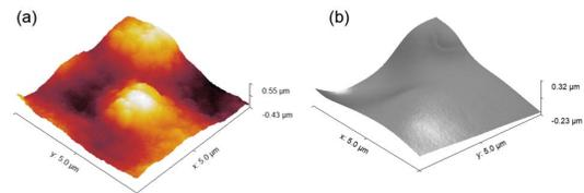
Fig. 6. AFM images of (a) the copper paste B sintered for 30 minutes at 260°C and (b) a reflowed solder paste.
