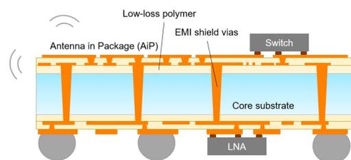
Fig. 1. Antenna-integrated packages with mm-wave chips assembled.
