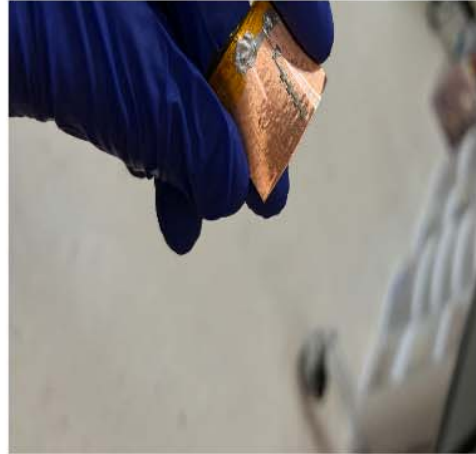
Figure 9: Flexible, inkjet printed RF Front-end of mmID tag.
