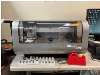
Figure 2. Inkjet printer used to print SU-8 and Suntronic ink.
