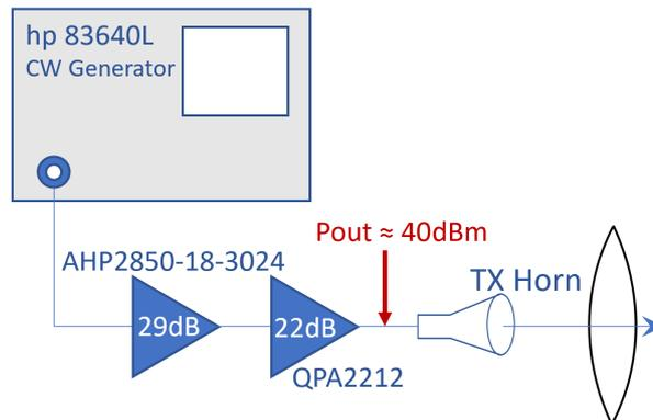
Fig. 4. Schematic describing the high performance transmitter setup.
