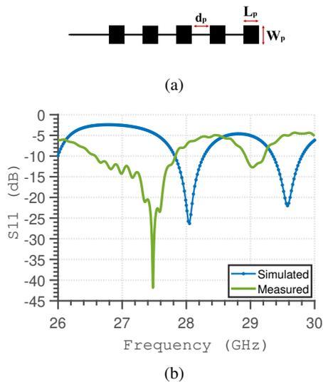
Fig. 1. (a) Schematic of the series-fed patch antenna array with  $W_p = 3.6\text{mm}$ ,  $L_p = 2.74\text{mm}$  and  $d_p = 2.8\text{mm}$ , (b) Plots of the simulated and measured  $S_{11}$  of the antenna array.
