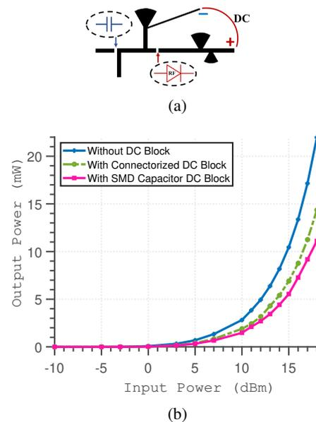
Fig. 2. (a) Schematic of the mm-wave rectifier with length  $L = 12\text{mm}$  and width  $W = 8\text{mm}$ , (b) Plots of the measured output powers vs input power of the rectifier with and without a DC Block for a load of  $980\ \Omega$ .
