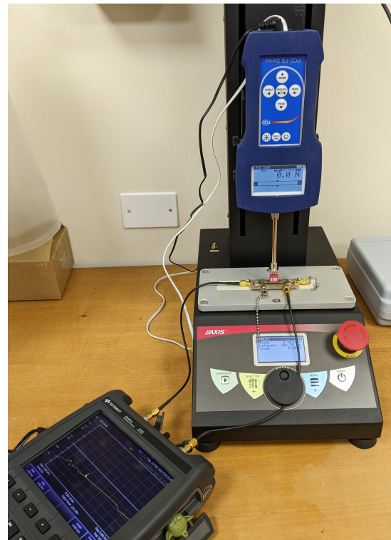
Fig. 5. Photo of the experimental setup used to test the proposed pressure transducer.
