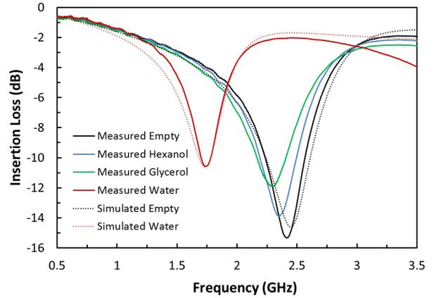
Fig. 5. Measured and simulated Insertion Loss (IL) for different fluids pumped into the channel.
