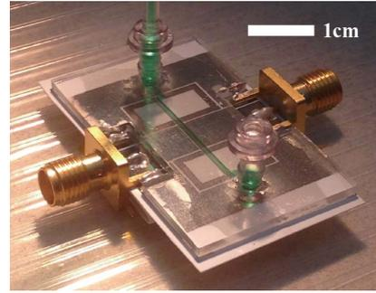
Fig. 3. Geometry (a) and photograph (b) of the proposed SRR bandstop filter.
