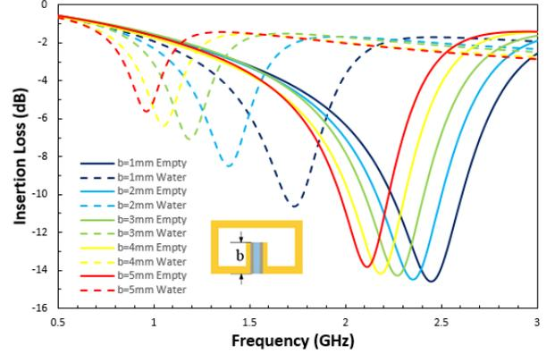
Fig. 4. Sensitivity change with different slot in simulation.
