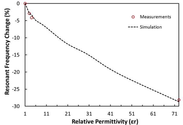
Fig. 6. Resonance frequency shift (in percentage) due to different fluids in the channel.
