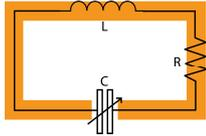
Fig. 2. Equivalent circuit of the SRR unit cell.
