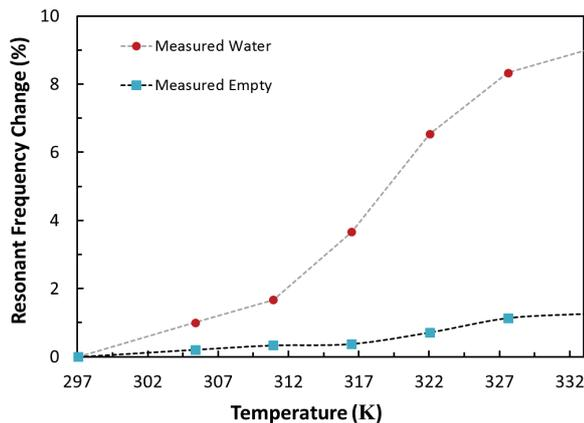
Fig. 7. Resonance frequency shift (in percentage) due to temperature change.
