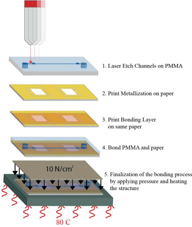
Fig. 1. Fabrication process.
