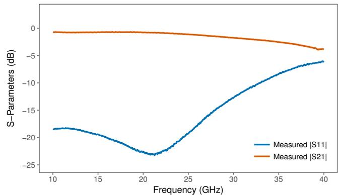
Fig. 3. Measured S-parameters for back-to-back inkjet-printed ramp interconnects with a 0 dB GaAs attenuator die on a MEG 6 laminate.
