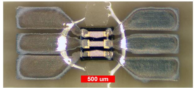
Fig. 2. Inkjet-printed ramp interconnects interfacing a Ka-band GaAs attenuator die.
