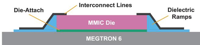
Fig. 1. 2D cross-section schematic of inkjet-printed ramp interconnects for a MMIC die on a MEG 6 substrate.
