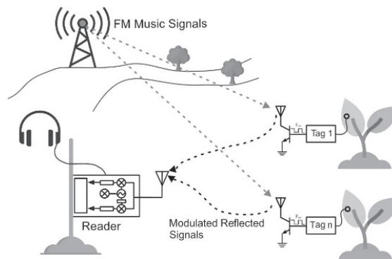
**Figure 1.** Backscatter communication using ambient Frequency Modulated (FM) signals. A commercial FM receiver can be used for collecting the data.
