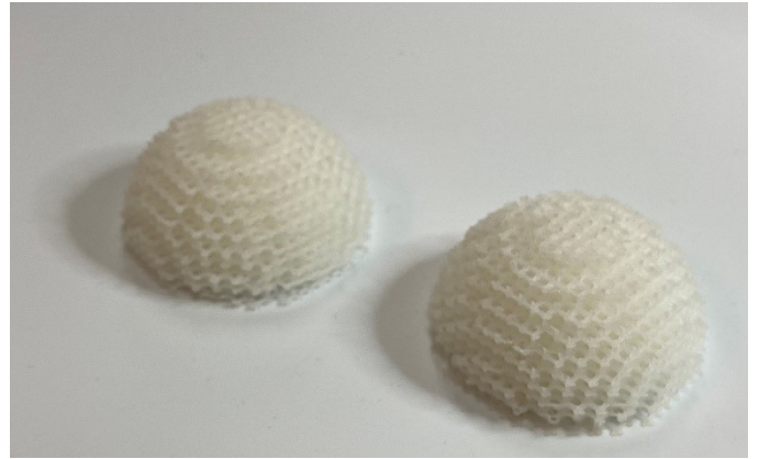
Fig. 6. Luneburg lens halves of 50 mm diameter with a 2.5 mm lattice constant FDM printed with ABS plastic.
