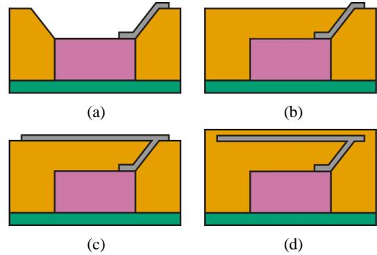
Fig. 7. Process flow outline of TMV integration with in-package structures: (a) partial encapsulation (orange) 3D-printed onto IC die (pink) and packaging substrate (green) with inkjet-printed sloped interconnects (grey), (b) encapsulation fill 3D-printed to seal package, (c) multilayer antenna/passive/etc. topology inkjet-printed onto encapsulation surface, (d) final encapsulation 3D-printed to finalize package.
