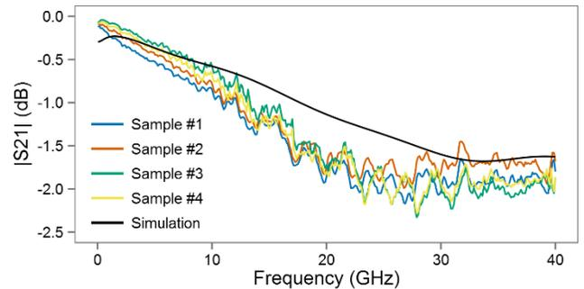
Fig. 4. Insertion loss simulation and measurements of inkjet-printed 3D interconnects. [7]
