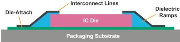
Fig. 2. Cross-section of inkjet-printed 3D interconnects. [7]
