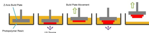
Fig. 1. Stereolithography (SLA) 3D printing process diagram.
