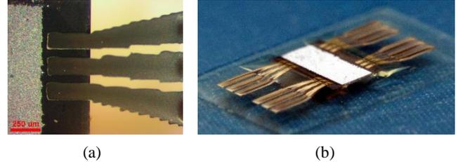
Fig. 3. Inkjet-printed 3D interconnects with die: (a) micrograph and (b) perspective view.
