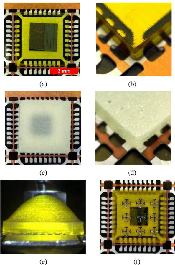
Fig. 5. 3D SLA-printed die encapsulations on a metallic QFN leadframe: Vorex encapsulation (a) top view and (b) perspective detail view; Porcelite encapsulation (c) top view and (d) perspective detail view; (e) Vorex dielectric lens structure; (f) Vorex encapsulation with inkjet-printed FSS. [13]
