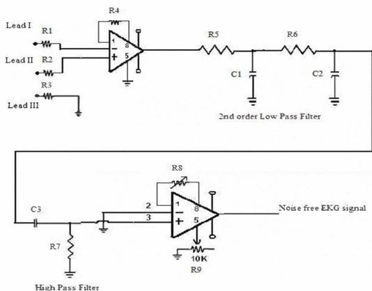
Fig. 2. EKG Acquisition Circuit
