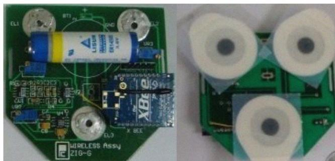
Fig. 4. Wireless EKG transmitter (Front and rear view)
