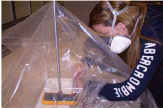
Fig. 4. The setting of Tedlar bag gas chamber for SWCNT gas reaction.
