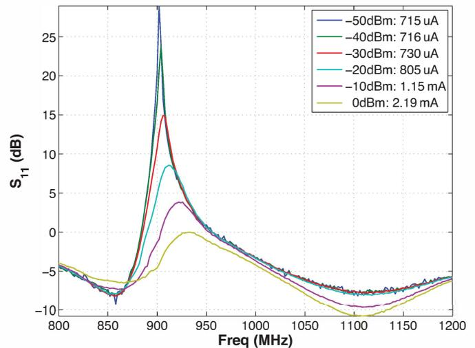
Fig. 6. Reflection amplifier gain as a function of the input power level.
