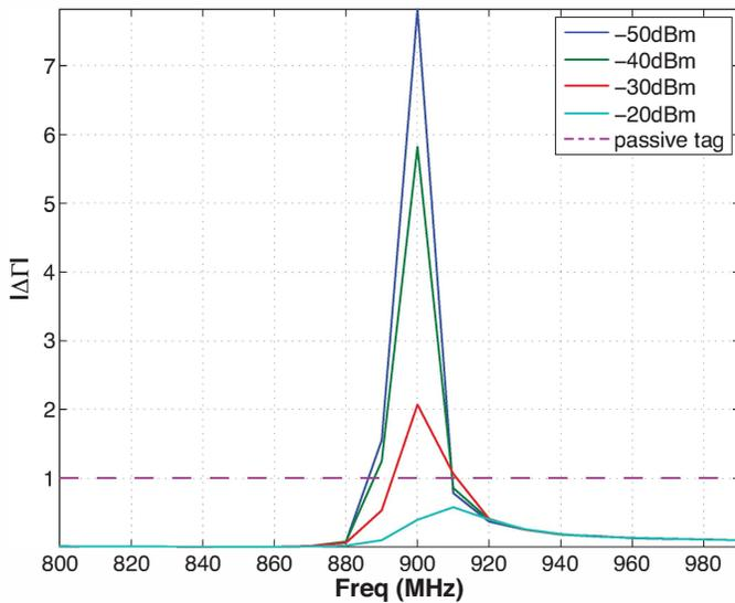
Fig. 8. Reflection coefficient difference amplitude as a function of the reflection amplifier input power level.
