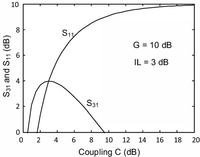
Fig. 2. Effect of coupling factor on system performance for amplifier gain  $G = 10$  dB.
