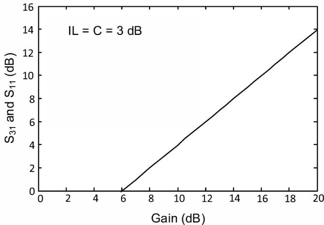
Fig. 3. Effect of amplifier gain on system performance for insertion loss and coupling factor equal to 3 dB.
