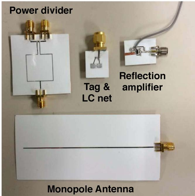
Fig. 4. Inkjet printed prototypes.
