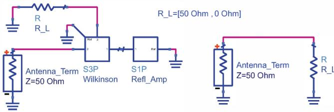
Fig. 7. Compared tag front-end models. Left: proposed system with reflection amplifier. Right: conventional tag.
