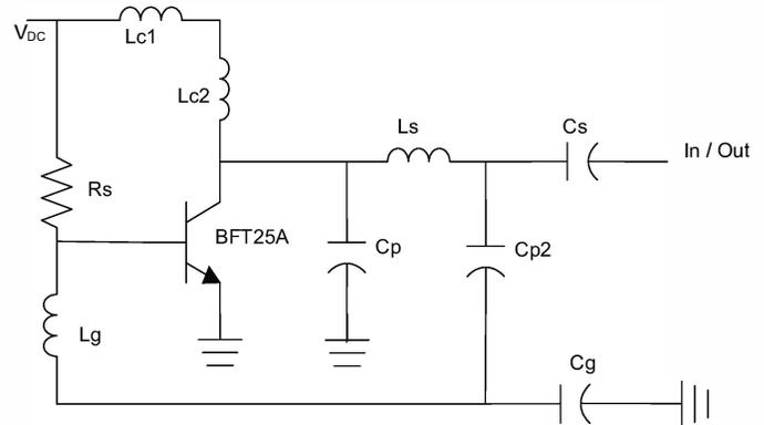
Fig. 5. Reflection amplifier circuit diagram.
