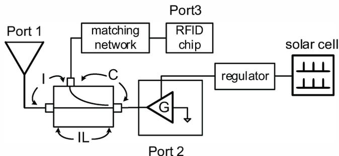
Fig. 1. Enhanced range passive RFID tag.
